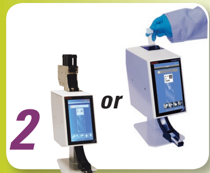
2. Place the slide into the printer or use the slide delivery system
