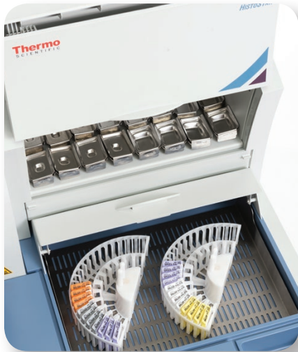
High-capacity tissue storage tank and mold storage
